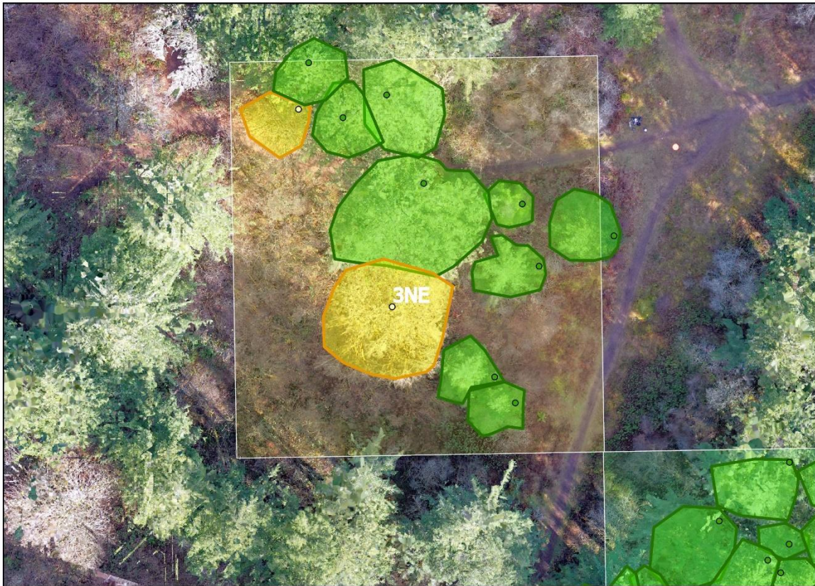
Figure 23: Example of the sample plots that have been manually segmented. Each tree crown has a polygon drawn around it and been coded by species.
