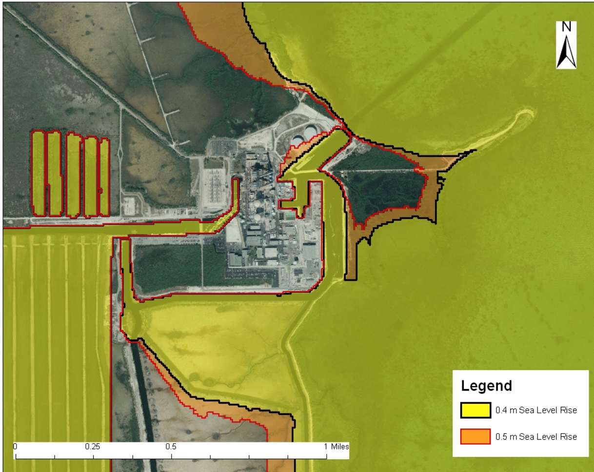
Figure 8. Turkey Point with a sea level rise of 0.4 m and 0.5 m.
