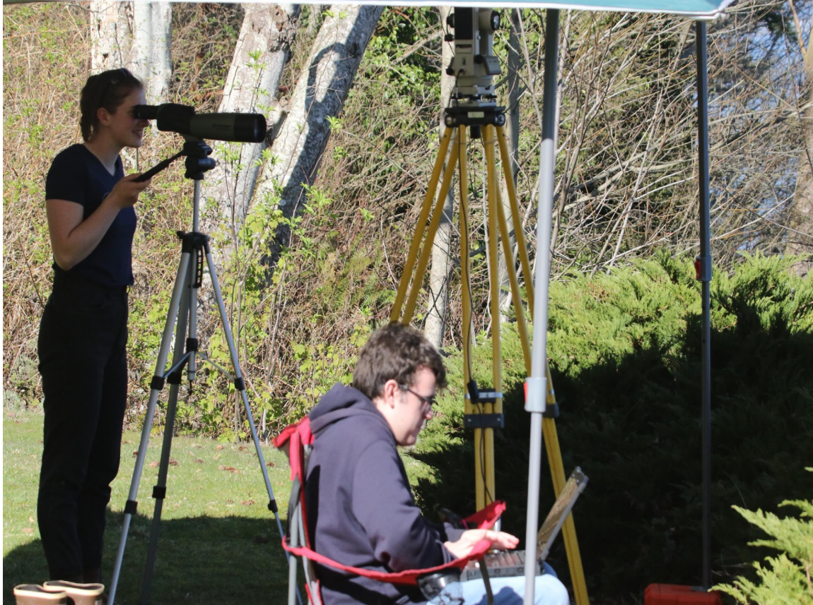
Figure 3-4: This image shows the team set up for tracking whales. The theodolite operator would be using the device on the yellow stand. The computer operator in the red chair would be recording the data. The spotter utilizing the spotting scope would be communicating data to the computer operator.
