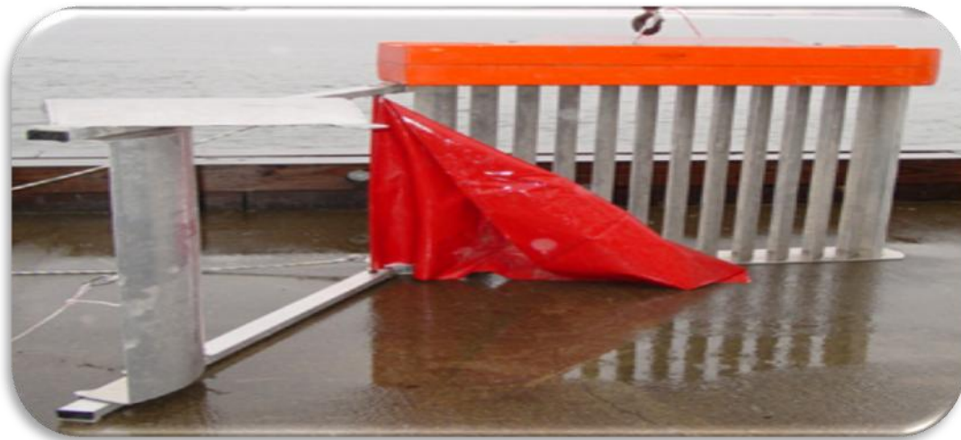
Figure 5. One-meter boom vane assembled for a deployment training exercise.
