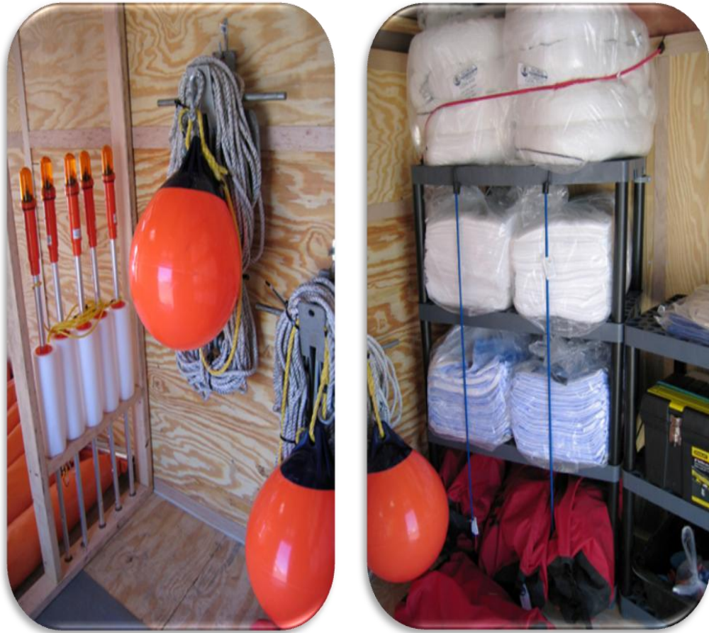
Figure 2. (Left) Anchor systems and navigation strobe lights.
