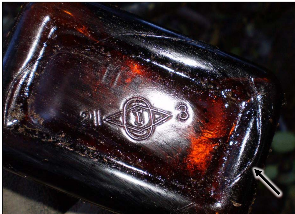
Figure 26. Example of bottle found at a historical camp site. This brown bottle was manufactured in 1933 based on the Owens-Illinois maker's mark shown. In the absence of a maker's mark, manufacturing variations can identify a possible production date. The oval-shaped seam on the bottom (indicated by arrow) is likely a cut-off scar where the bottle was cut from a suction machine; this type of scar dates the bottle between 1904 and 1950. Photograph by author (Ferguson, 2011A).
