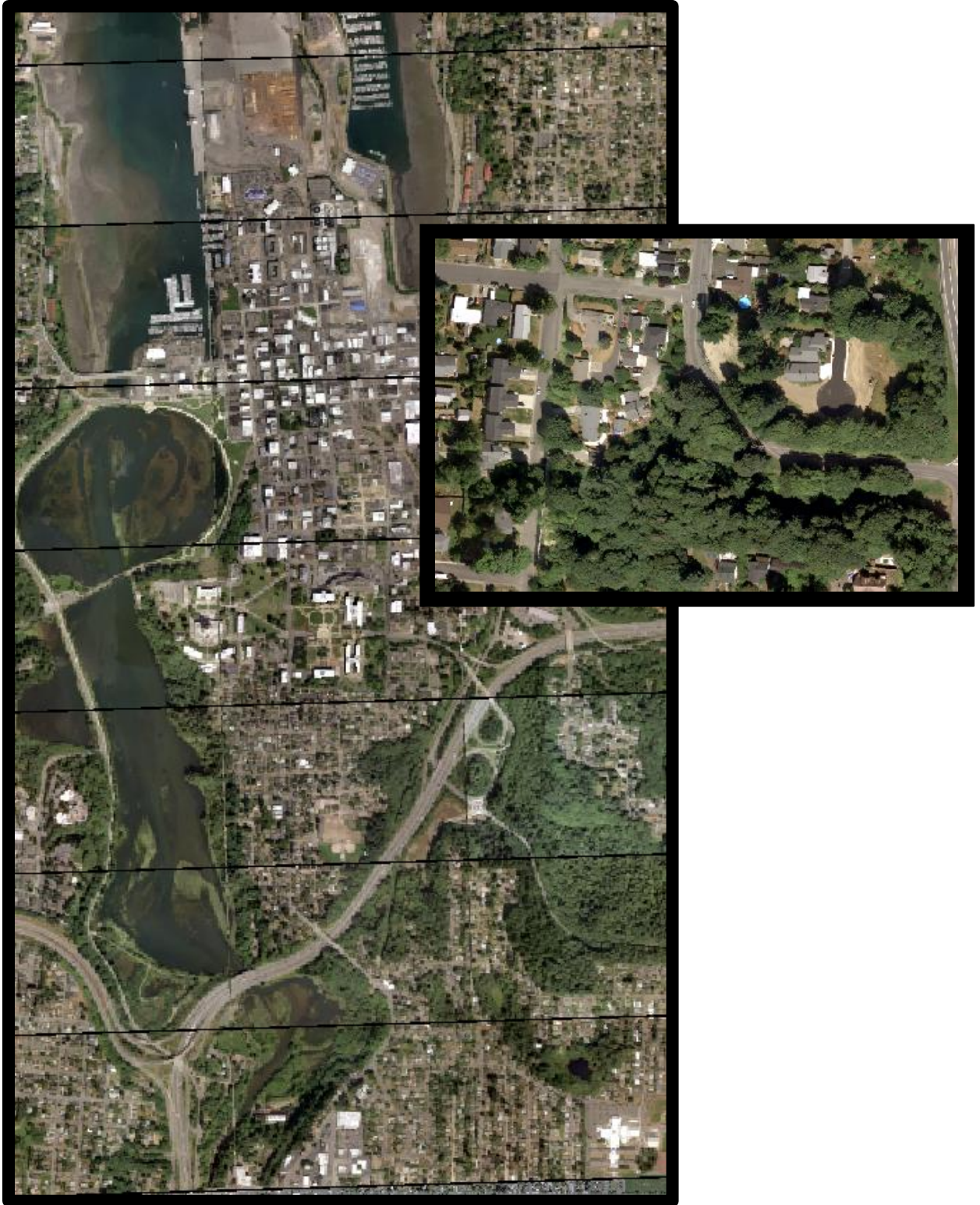
Figure 11. 2008 high-intensity orthoimagery, 1.5 Foot GeoTiffs, Datum NAD1983. Inset example demonstrates magnification capability for analysis.
