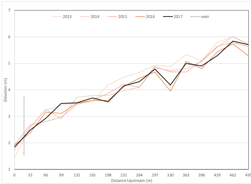
Figure 24A. Changes in the thalweg profile of sub-reach 1 (stations 3-18) at lower BBC, 2013-2017. The location and elevation of the weir is indicated by the vertical dashed line. The observable decrease in thalweg elevation at 330m (station 13) was associated with a large/deep pool created when a buried log re-emerged from the channel bed. Phase 2 wood structures were placed within the uppermost portion of this reach ( \geq 429\text{m} ) in 2016.
