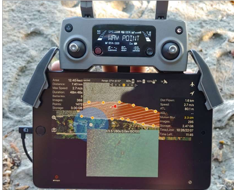
Figure 13. View of Map Pilot automated survey grid generated for survey at North Beach County Park. Photo credit: Tyler Cowdrey
