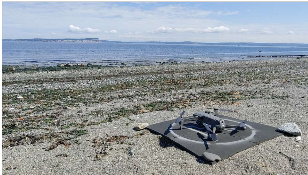
Figure 12. DJI Mavic 2 Pro on the launch pad prior to a survey in Hansville, WA. Photo credit: Tyler Cowdrey
