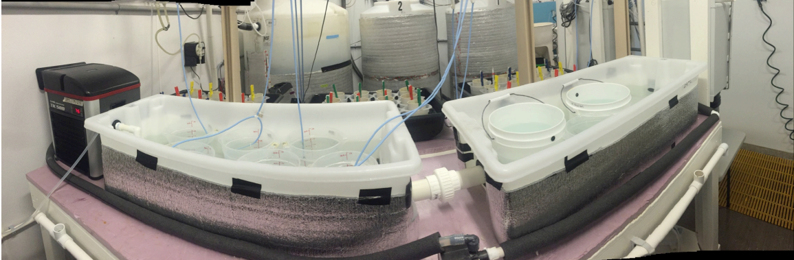
Figure 19. Photograph of the 24°C system without the lids. The first tote (left) connected directly to the inflow from the Teco TK500 chiller and contained the six experimental replicates. The second tote (right) contained three 2 gallon buckets filled with clean water for future water changes. The freshwater flowed out from the right tote the external pump (pictured in the bottom center), which pumped directly back to the chiller. Photo Credit: Kendra Baird.
