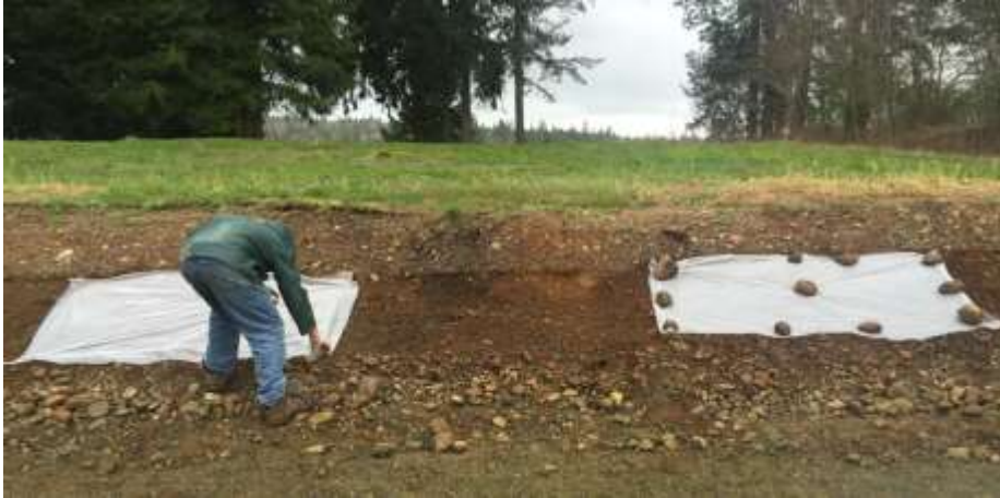
Figure 3.1 Affixing polyethylene sheeting to plots during seeding preparation.
