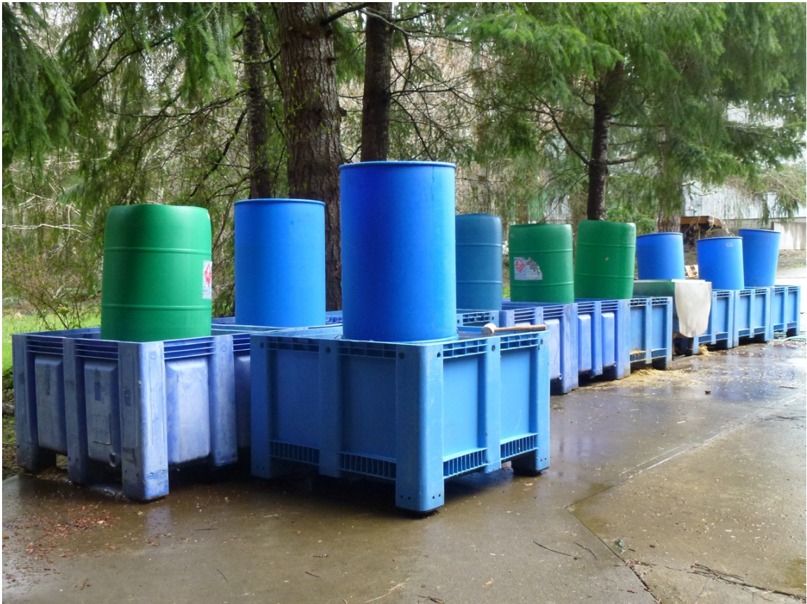
Figure 33: Ambient Temperature (40-60 F.) Fermentation of Woodchips in Fresh Water
