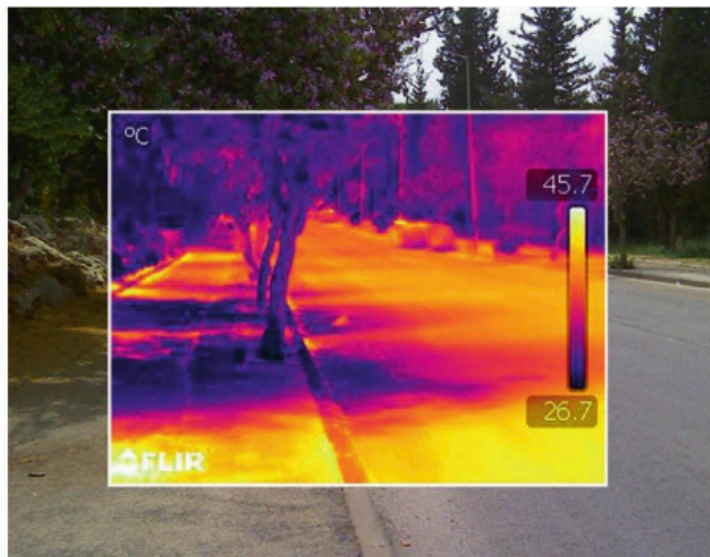
Figure 2. Thermal infrared image indicating the daytime difference in radiative surface temperature between exposed and tree-shaded pavement. (Pearlmutter et al., 2017)
