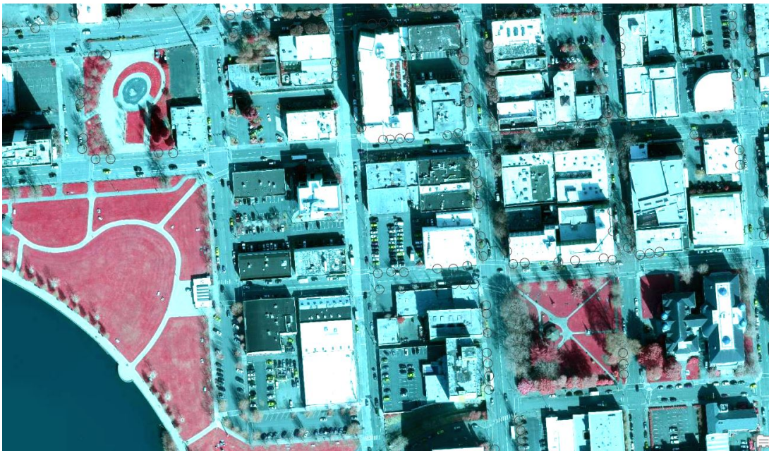
Figure 30. NDVI analysis using aerial imagery of Downtown Olympia in winter, showing red chlorophyll response of grass and conifer trees, but no response from street trees (circled in black).
