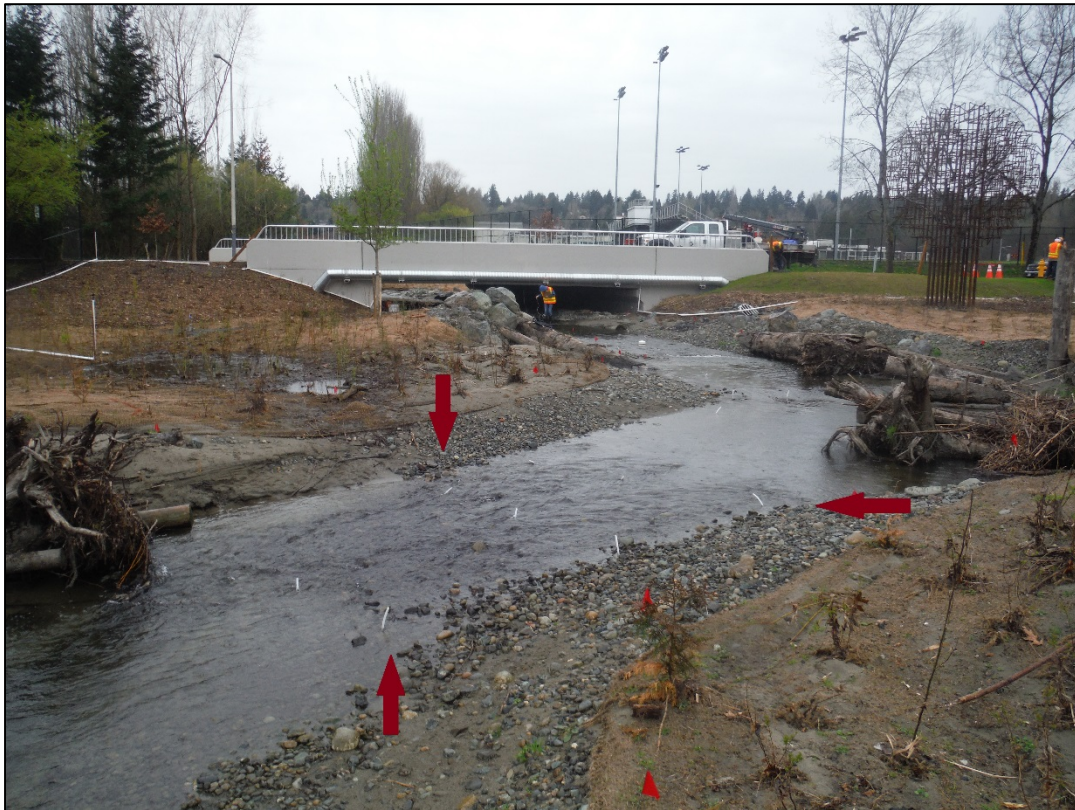
Figure 6: Photograph of South Fork Confluence treatment (downstream) study site. Shows the characteristic transect and tube arrangement used for all six surveys. The photograph shows transects placed at the upstream, middle, and downstream section of a riffle unit.
