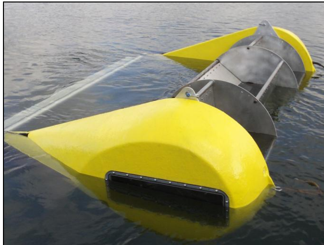
Figure 7: A C2 Canal Turbine equipped with Darrieus rotor blades
