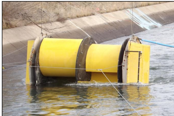
Figure 2: The C3 Prototype Turbine being lowered into Roza Canal
