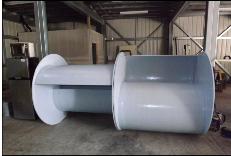
Figure 8: A Turbine with Savonius rotor blades
