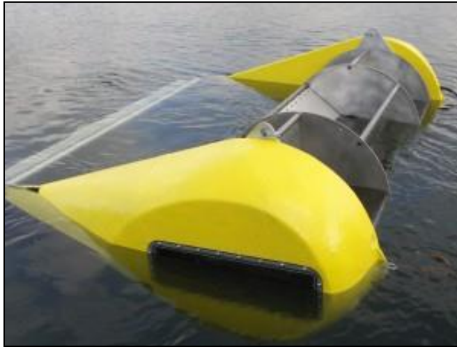
Figure 4: The C2 Canal Turbine
