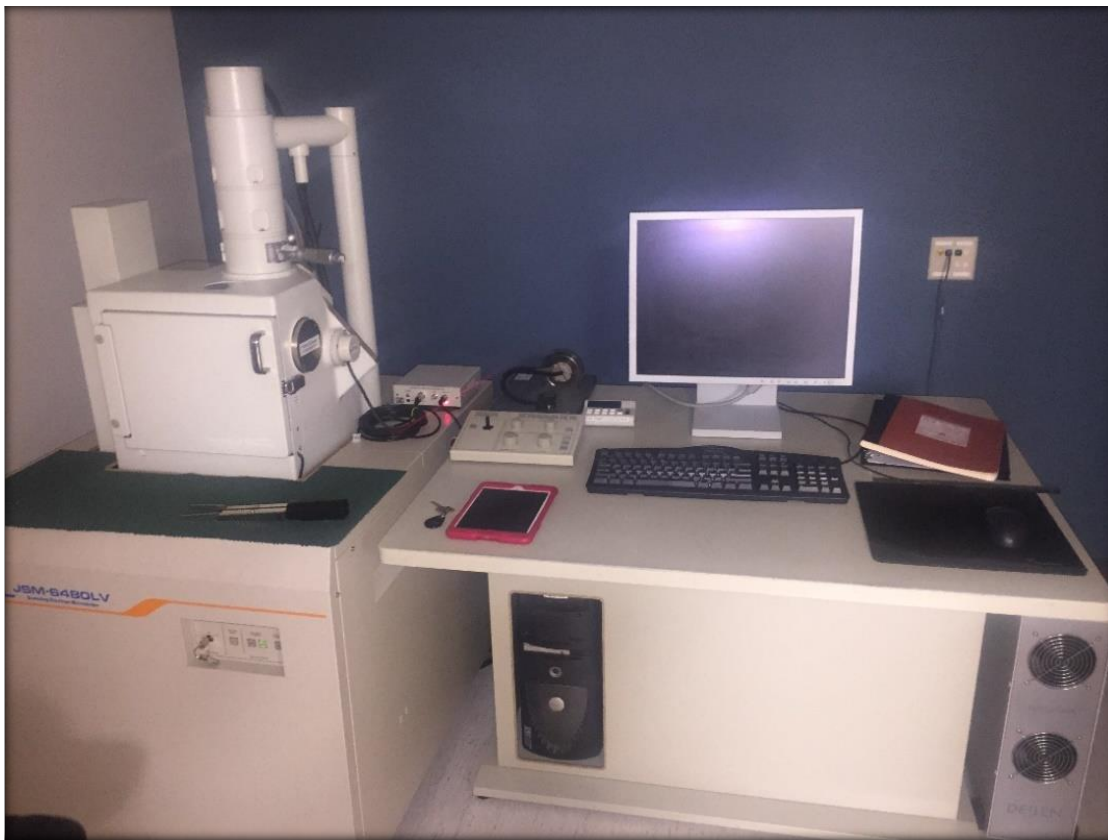
Figure 6. Image of The Evergreen State College's Scanning Electron Microscope. Model JEOL JSM-6480LV. To the left is the microscope and to the right is the computer monitor with SEM control panel between them.
