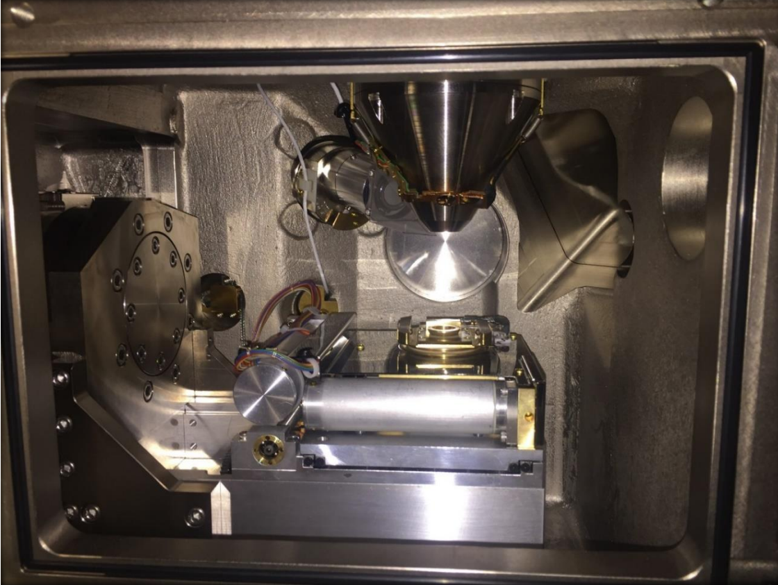
Figure 7. Image of The Evergreen State College Scanning Electron Microscope sample chamber.
