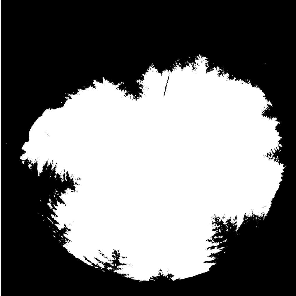
Figure 18: Manually thresholded image of Figure 17. When thresholded this becomes a black and white record of sky obstruction. When the image from this search plot was processed through Gap Light Analysis 60% of the canopy is open but that underestimates the amount of sunlight the plot gets because of its slope, aspect and where trees block the sun. Total direct sunlight reaches this plot is 90.4% of the time. North is at the top of photo.
