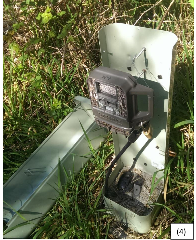
Note: Forms of camera installation: (1) Telespar; (2) Tree Mount; (3) Utility Box (Exterior); (4) Utility Box (Interior)
